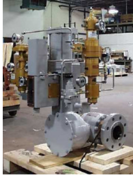
Figure 8.0– Becker VRP-SB-PID Controller on RPDA Series Actuator and HPP Series Positioner
